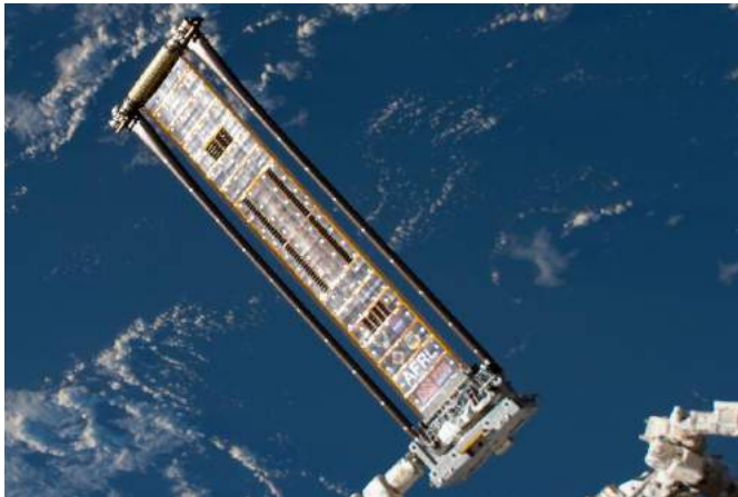
Roll-out solar array (AFRL, NASA, and DSS)
